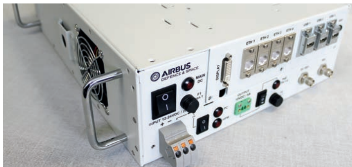
Left: Airbus Defence and Space's standalone Tactilon Cell can be used to create a small LTE network. It comprises a base station, terminals, LTE software and an app server for mission-specific apps. All the cell's features comply with 3GPP standards. Right: the recently launched Dabat integrates a complete TETRA radio and smartphone in one device. Airbus says it can work on any TETRA network.
